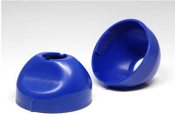
This cap is designed to fit on the injection pump type 80394K and makes it possible to empty the FiloSlim resin bags up to 400ml with use of the injection pump.
