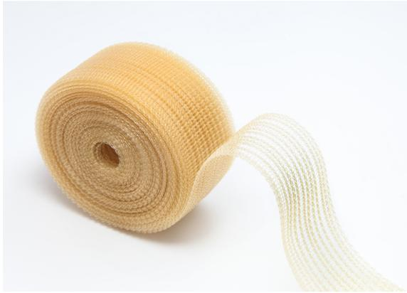
This polyester gauze is used to create sufficient insulation distance between the conducting parts within the injection joint. Furthermore the gauze contributes to a proper flow of the resin into the joint.
