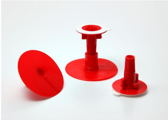
Filoform injection nipples and injection valves are used for injection joints. The injection valve is positioned on the wrap-around gauze by using the wrap-around tape. The injection nipple is placed onto the resin pack in order to enable an easy and smooth injection of the resin into the joint. Recommended for injection joints on cables
