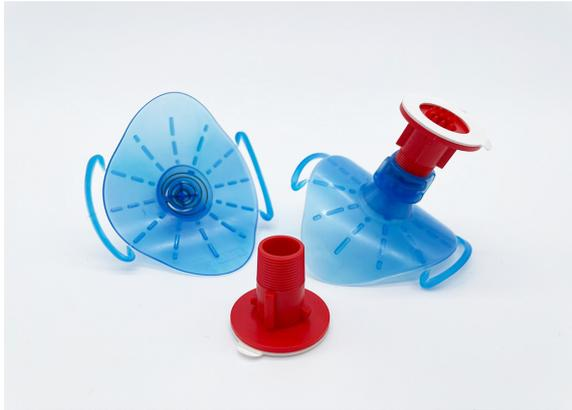
Filoform injection nipples and injection valves are used for injection joints. The injection valve is positioned on the wrap-around gauze by using the wrap-around tape. The injection nipple is placed onto the resin pack in order to enable an easy and smooth injection of the resin into the joint. Recommended for injection joints on cables  $>4 \times 25 \text{mm}^2$
