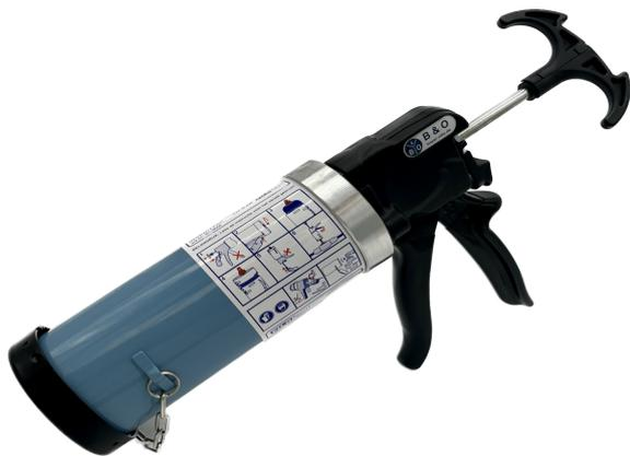
The new Filoform injection pumps GN-E5 are used to pump the resin under pressure ( $\pm 2$  Bar) into injection joints. The injection pump has a continuously variable piston displacement enabling an optimal flow of the resin into the joint.
