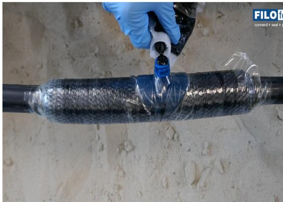
The FILOSLIM Sheath Repair Kit utilizes a totally enclosed mix-and-pour polyurethane resin technology, designed for use as a permanent repair of damaged cable sheaths.
