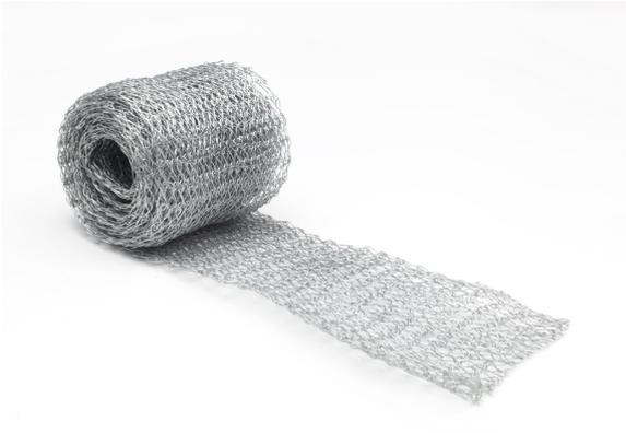
Filoform steel wire mesh is a knitted wire mesh of tin-plated steel wire and is used for EMC-shielding and continuation of the earth connection in joints for signalisation cables.
