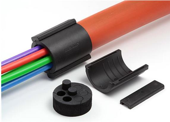
Suitable for gas and watertight sealing of 50mm HDPE ducts, which contain mini ducts and / or (fibre optic) cables. The modular system will guarantee easy installation of various different cable and duct configurations. Our system is divisible so can be applied at installation or afterwards. The rubber inserts can be custom designed for your specific needs and configuration and will contain (temporary) blind plugs to make the system more flexible at the installation site.
