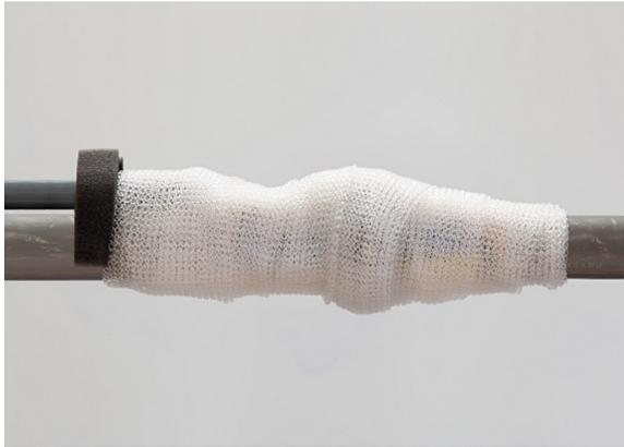
FiloSlim 3D Gauze Rolls are used for the construction of the FiloSlim cable joints. Thanks to the special 3D weave of the gauze, optimal insulation distance is created with just a few wraps.
