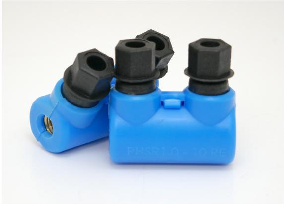
Suitable for making a safe connection of live cables without stripping the insulation from the conductor. The connector is completely safe to touch during the installation. The connector can be installed without stripping the conductors. An independent assembly thanks to the plastic shear bolt. The insulated connector is safe in use.
