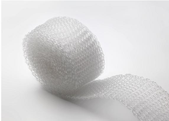
FiloSlim 3D Gauze rolls are used for the construction of the FiloSlim cable joints or the Taped resin injection joint. Thanks to the special 3D weave of the gauze, optimal insulation distance is created with just a few wraps.
